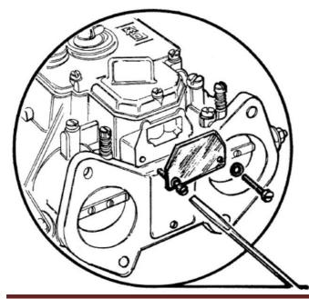
Carburetor mod. 42 DCOE 12 and 45 DCOE 12 are not fitted with starters so the housing space is closed by a metal plate
