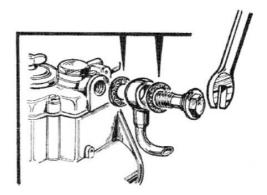
On re-assembling, carried out by inverting the above procedure, check the state of gaskets and the flat surfaces for perfect sealing before connecting fuel pipe.
